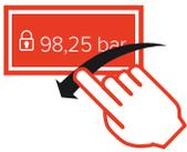
Using the TFT touch-screen, 2 PNP switching outputs can be set quickly and conveniently with a virtual scroll wheel.
